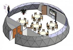
Geodesic Dome Classrooms: a geodesic dome is a is a hemispherical thin-shell structure (lattice-shell) based on a geodesic polyhedron. The triangular elements of the dome are structurally rigid and distribute the structural stress throughout the structure, making geodesic domes able to withstand very heavy loads for their size.
